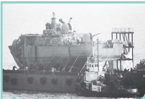
The South Korean corvette Cheonan being salvaged after having been sunk by a North Korean torpedo attack
